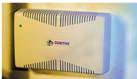
Figura 11. Detalle de la pasarela Coactive Conector 2000 series. Fuente Coactive Networks.
